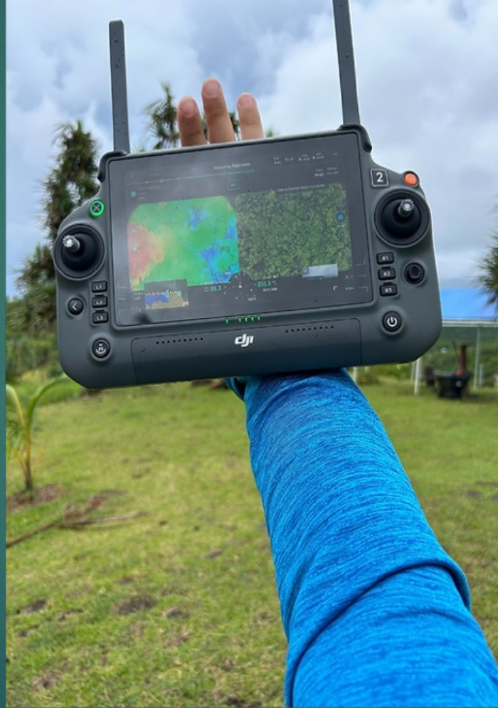
DJI RC Plus controller with a Side by Side view of the LiDAR capturing data
